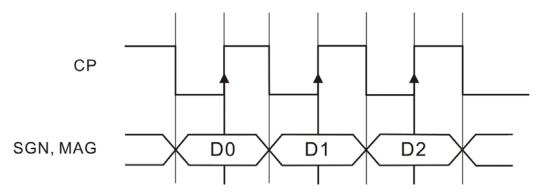
For the PT9120, the CP pin may be used as either clock input or output. With the on-chip reference crystal oscillator enabled, the CP pin becomes an output and delivers a CMOS-level signal with a nominal duty cycle of 50% at the same frequency as the reference crystal oscillator. By disabling the on-chip crystal oscillator (setting XEN to logic LOW), the CP pin becomes an input which accepts an external CMOS-level (TVSS to TVDD) clock signal with a duty cycle between 40% and 60%.
